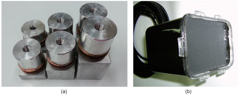
Fig. 1. Photographs of the 6 tonpiliz transducer elements operating at different resonance frequencies (a) and the multi-resonant broadband acoustic transducer (b) developed in this study. The transducer elements were arranged in a 2×3 array configuration on the acoustic window of polyurethane.
